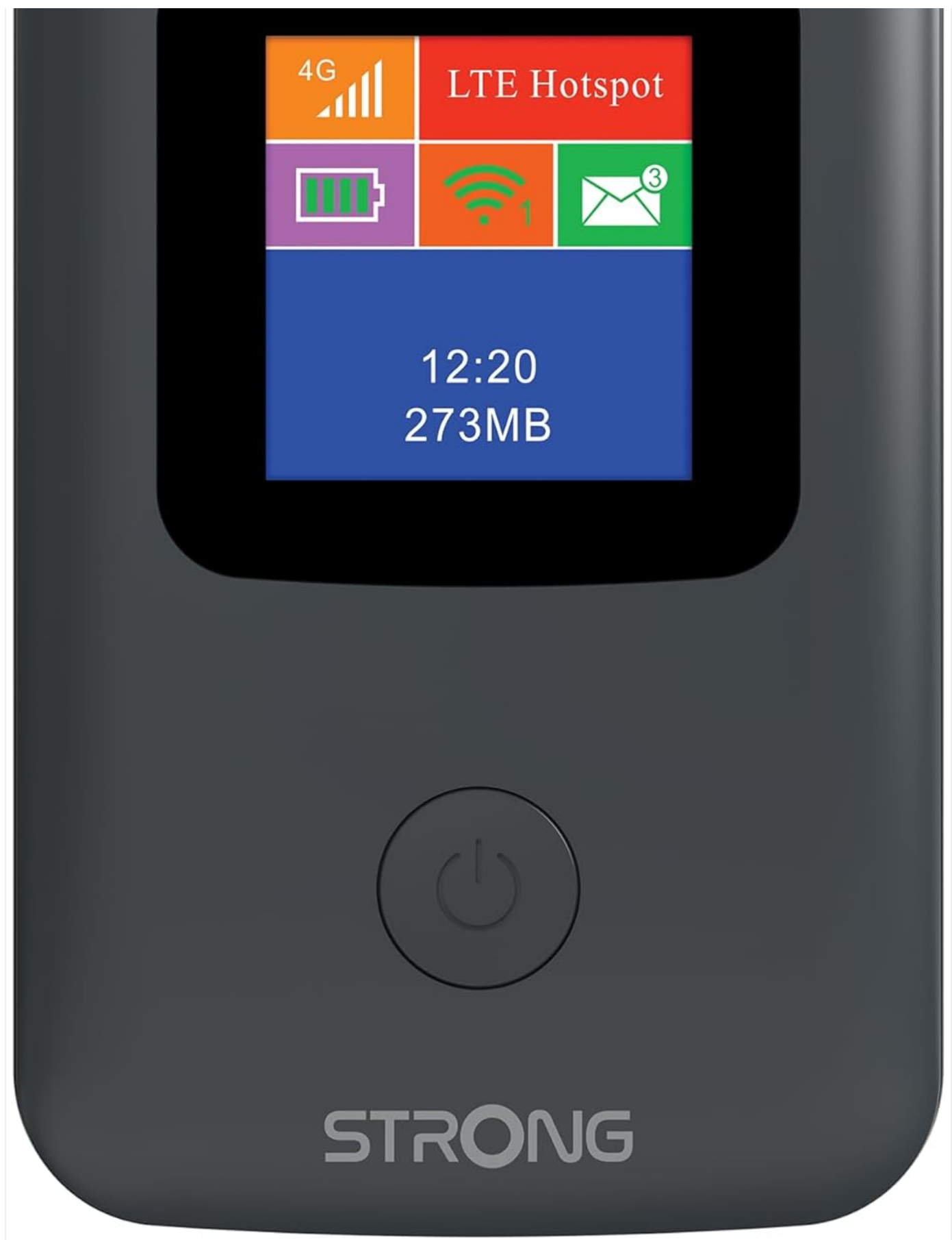
Image: Front view of the STRONG 4GMIFI150D Mobile Hotspot. It features a central display screen and a power button below it. The screen shows indicators for 4G signal, LTE Hotspot status, battery level, Wi-Fi signal, SMS reception, current time, and data usage.
