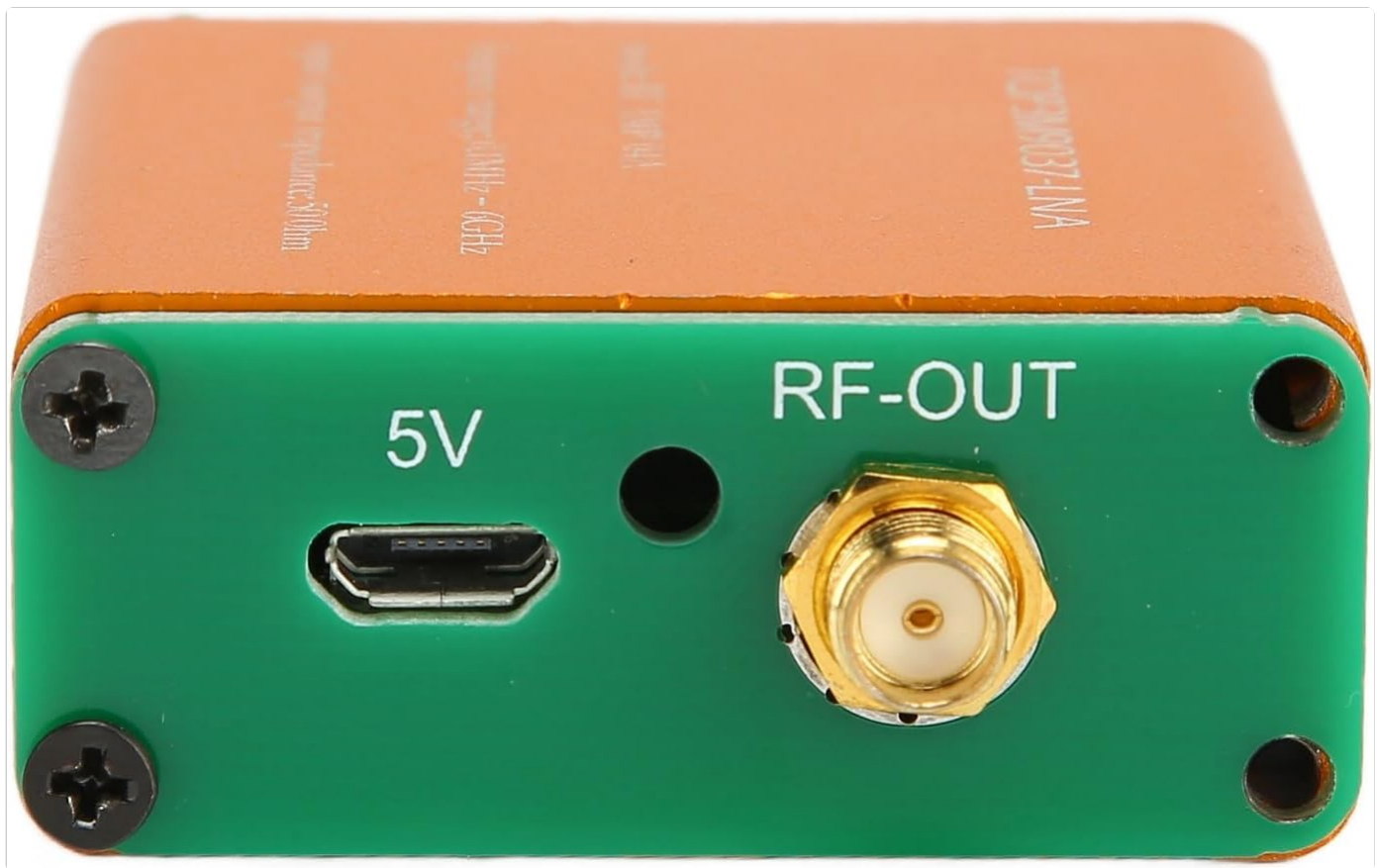
Figure 2: Rear view of the ASHATA LNA Module, showing the RF-OUT connector and power input.
