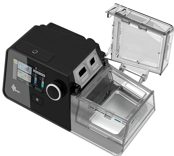
Figure 2: The BMC G3 A20 device with its integrated humidifier chamber opened, revealing the water reservoir for humidification.
