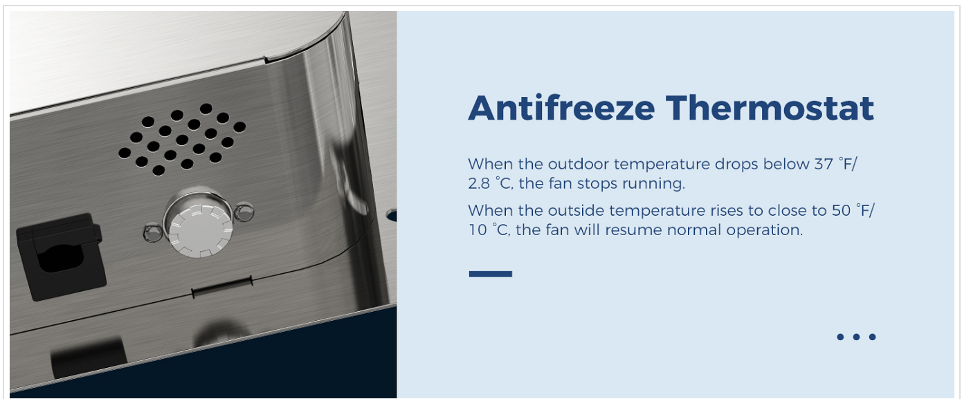
Image 7.2: Detail of the antifreeze thermostat.
