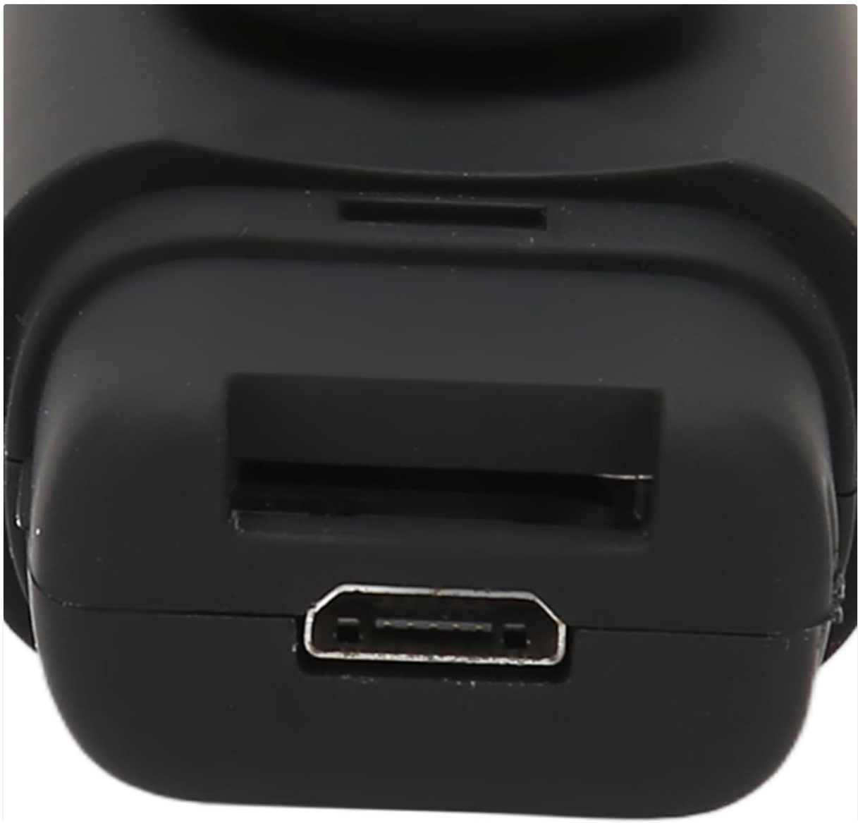
Figure 4: Camera USB Port. This image shows the Micro USB port located on the camera, used for charging and connecting to a computer.
