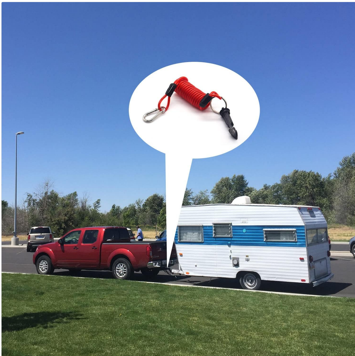
Figure 4: Proper connection of the breakaway cable during towing.
