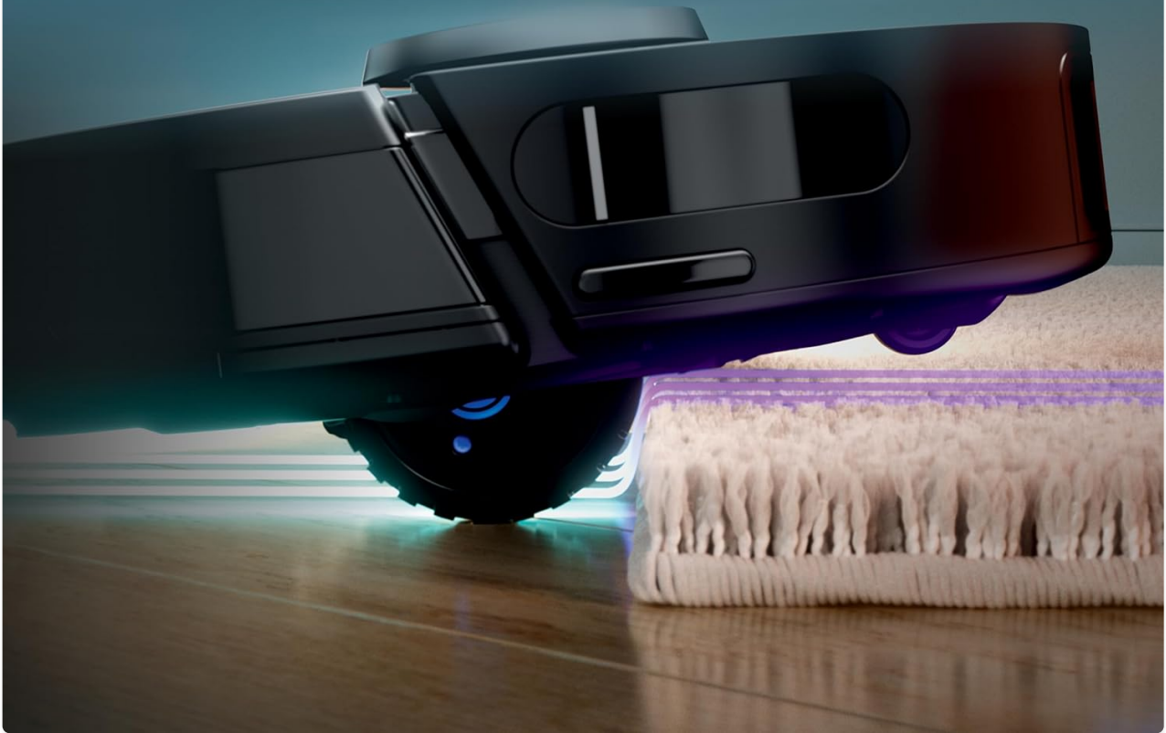
Image: The robot vacuum demonstrating its Active Lift & Lower feature, raising its body to easily move over a thick rug from a hard floor.
