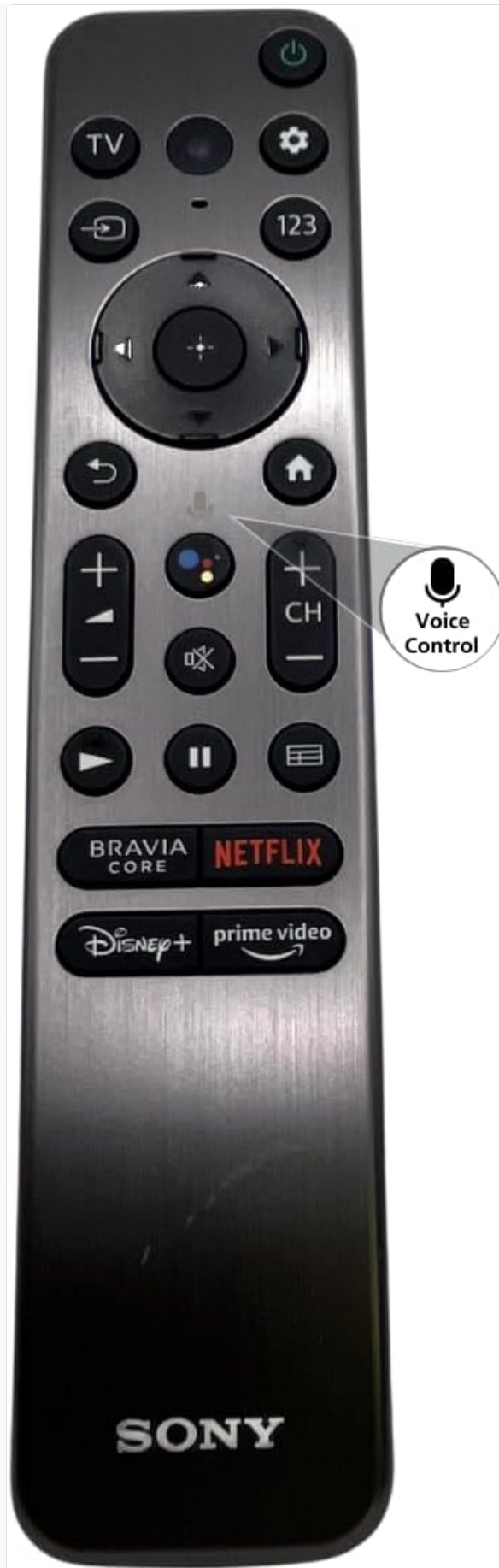
Figure 2: RMF-TX900U remote control with an overlay pointing to the voice control button. This image specifically highlights the microphone icon button located below the navigation pad, indicating its function for voice commands.
