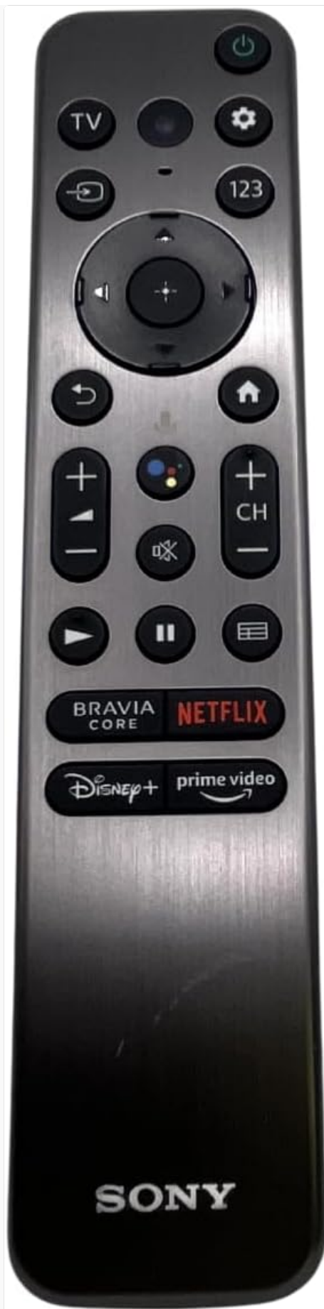
Figure 1: Front view of the RMF-TX900U remote control. This image displays the full button layout, including power, TV, settings, number pad, navigation, volume, channel, playback controls, and dedicated app buttons for BRAVIA CORE, Netflix, Disney+, and Prime Video. The remote has a dark, brushed metal appearance.
