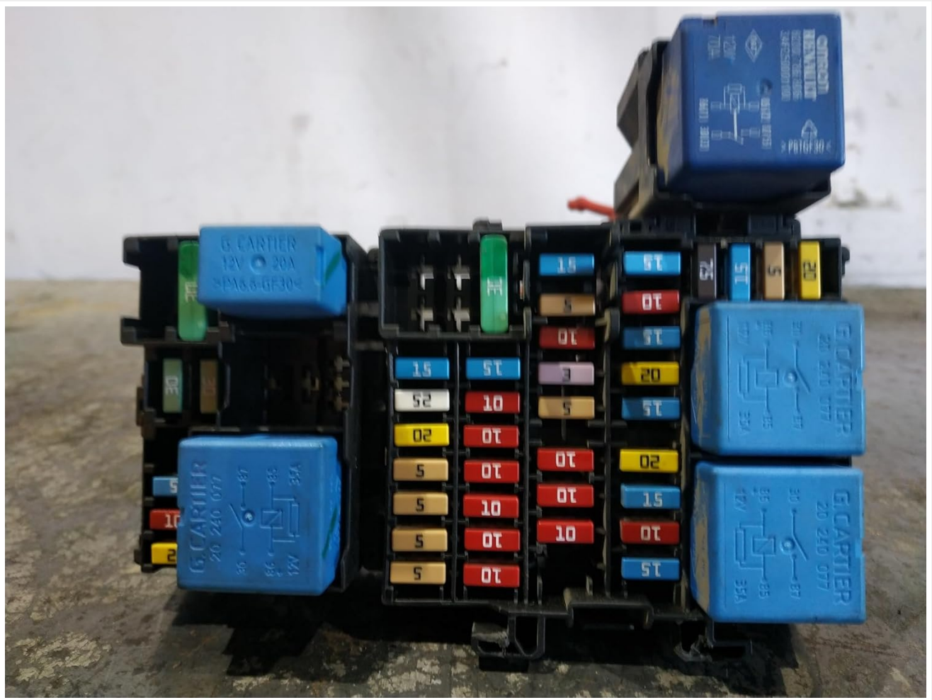
Figure 2.2: Angled view of the relay/fuse box. This perspective provides a closer look at the individual relays and fuses, allowing for better identification of their types and positions within the box. Some relays are labeled "G. CARTIER 12V 20A".
