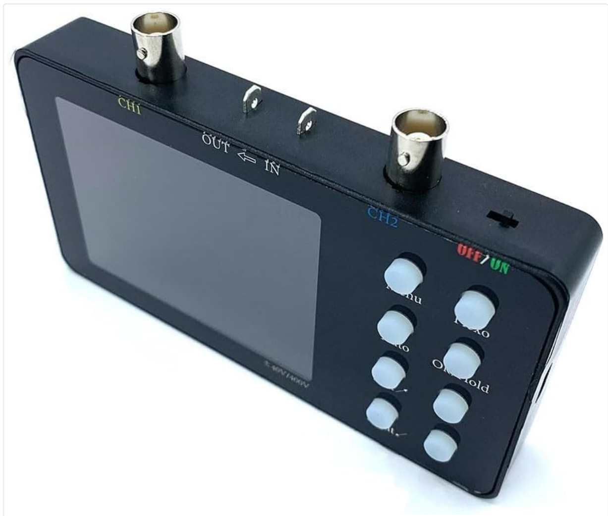
Figure 2.1: Angled view of the oscilloscope, highlighting the BNC input connectors for CH1 and CH2, and the power button.
