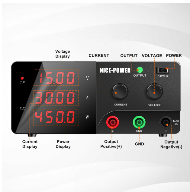
Figure 2: Detailed view of the front panel, highlighting the 4-digit LED displays for Voltage, Current, and Power, along with the Current and Voltage adjustment knobs, Output switch, and Power button. Front terminals are clearly marked for positive (+), ground (GND), and negative (-) with a 5A max rating.
