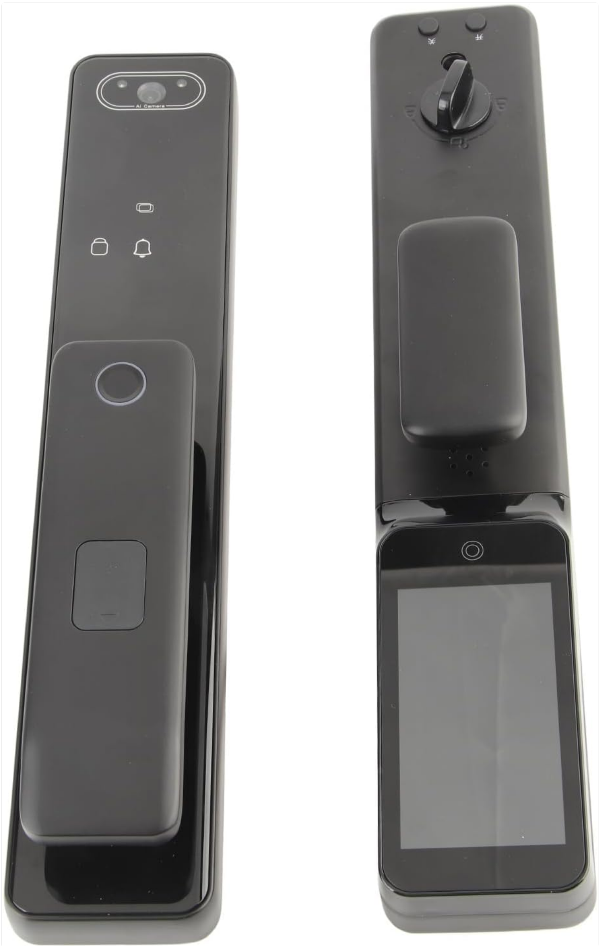
Image 3: Internal and external units of the smart lock.
