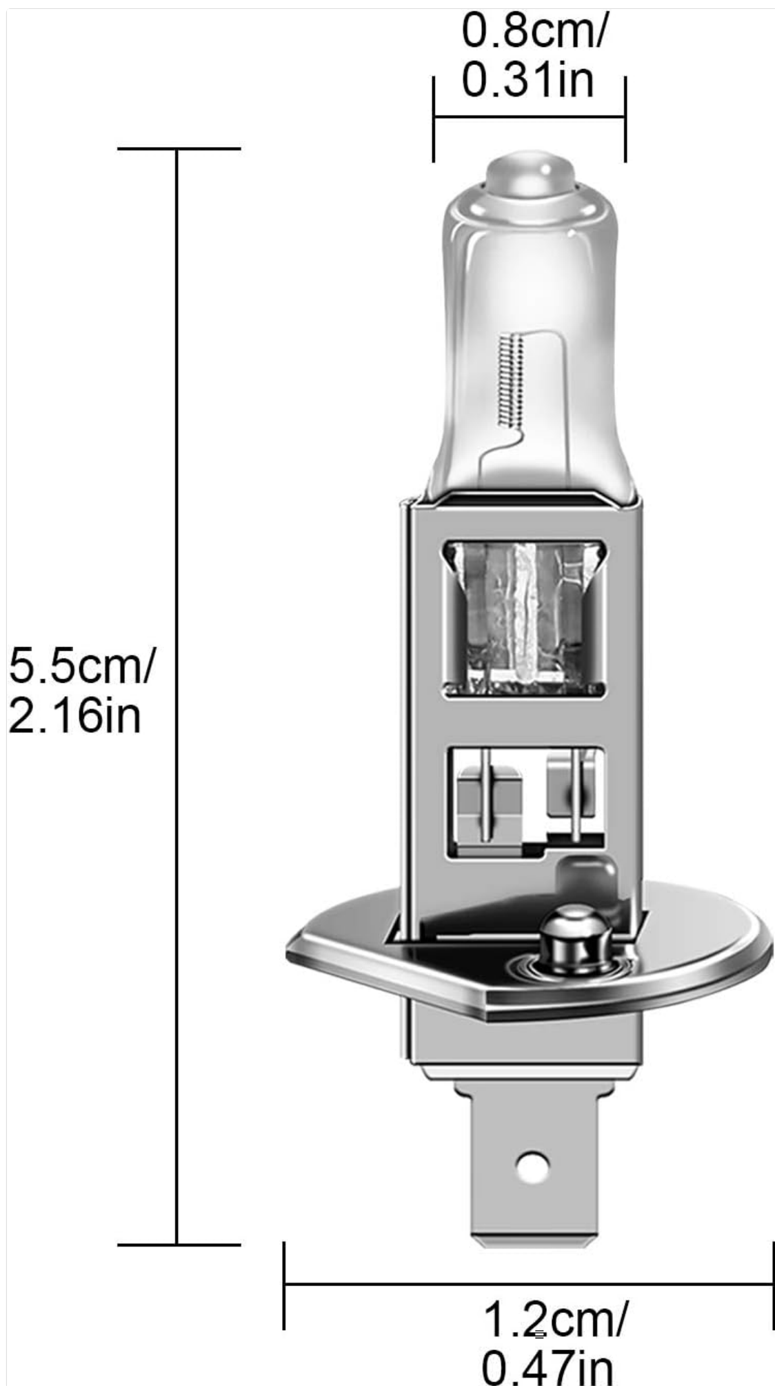
Image: Dimensions diagram of the H1 Halogen Headlight Bulb (approx. 5.5cm/2.16in length).
