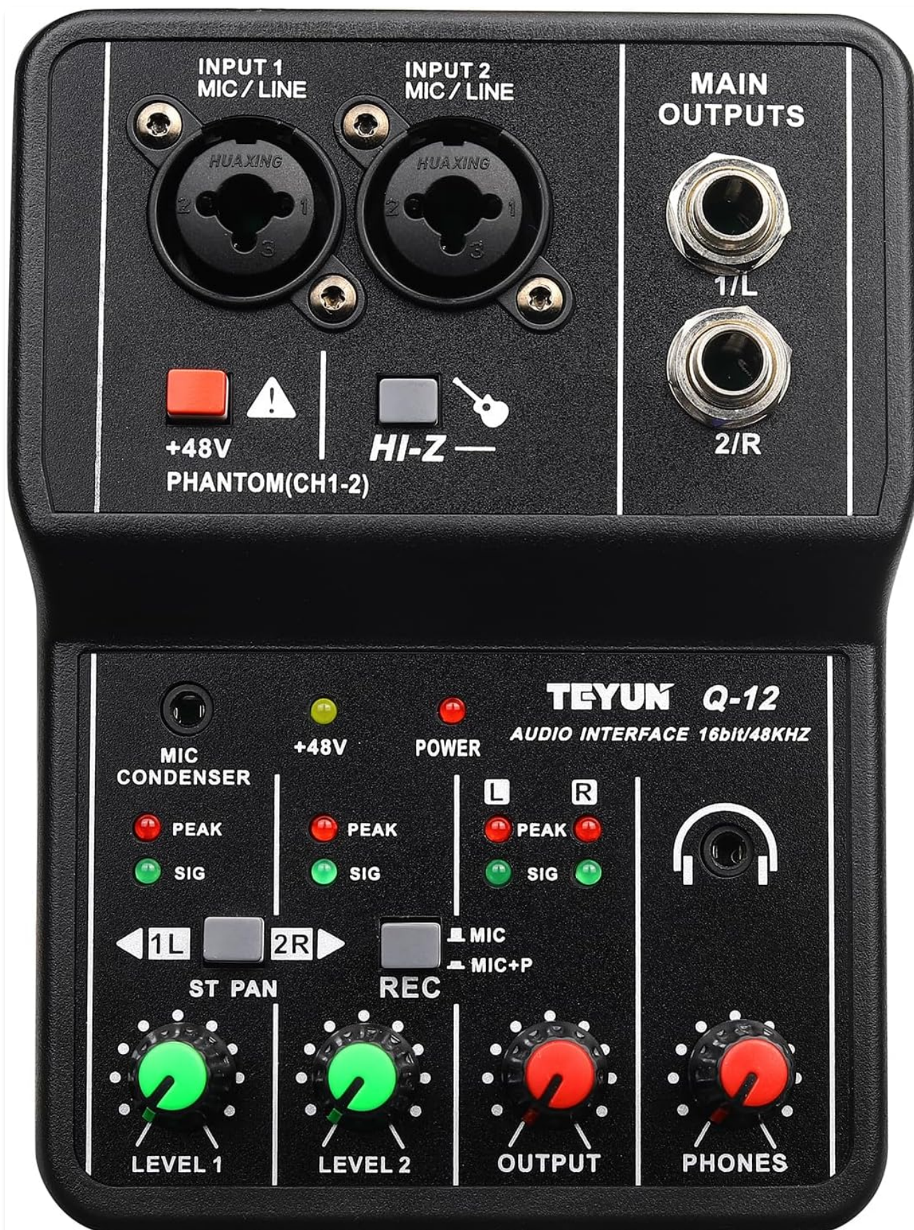
Figure 1.1: Front view of the TEYUN Q-12 USB Audio Interface.
