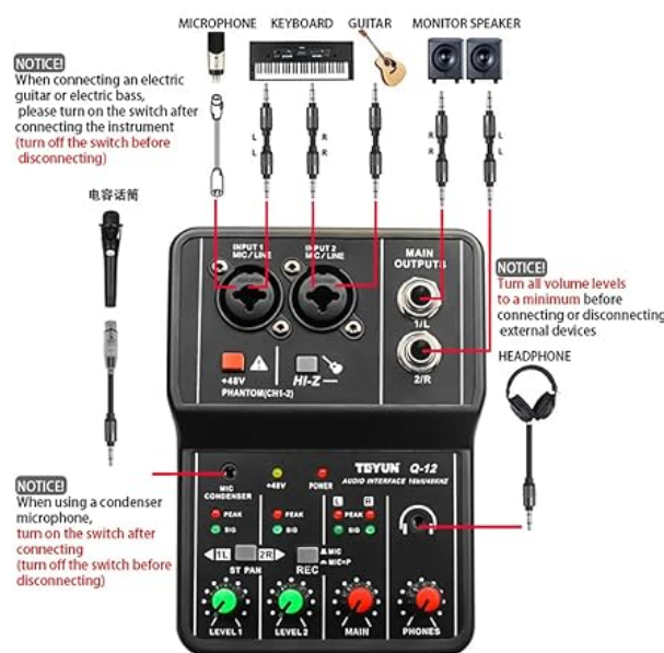
Figure 4.1: Diagram illustrating typical connection setups for the TEYUN Q-12.
