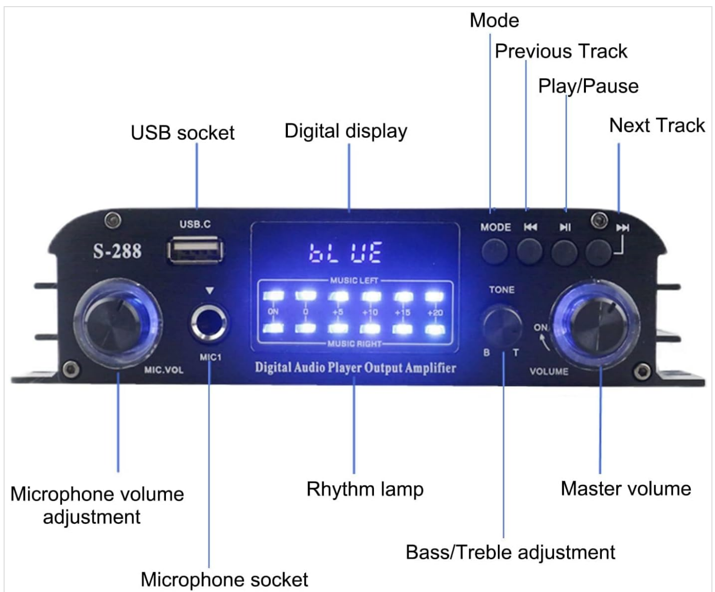
Figure 2: Front Panel Layout of the Romicta S-288 Amplifier.
