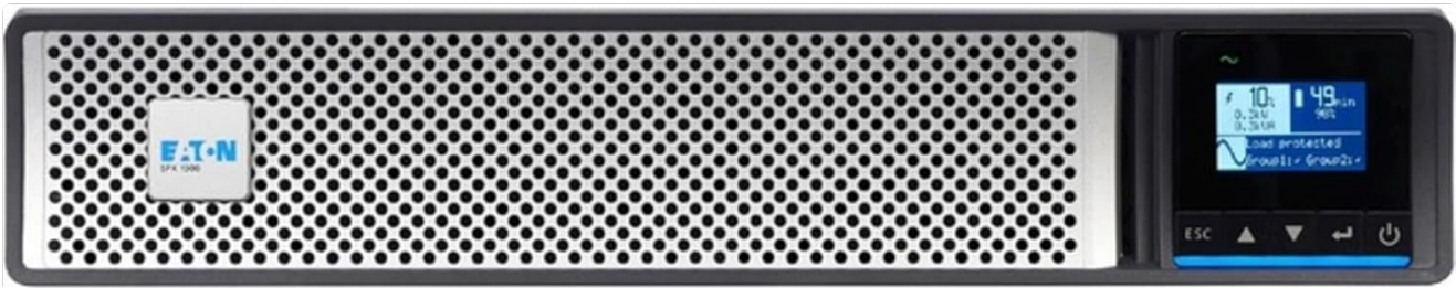
Figure 1: Front panel of the Eaton 5PX G2 Uninterruptible Power Supply. The left side features a perforated metal grille with the Eaton logo for ventilation. The right side houses a digital display showing operational status, including battery charge level, current load percentage, and estimated battery runtime. Below the display are control buttons for navigation and power management.
