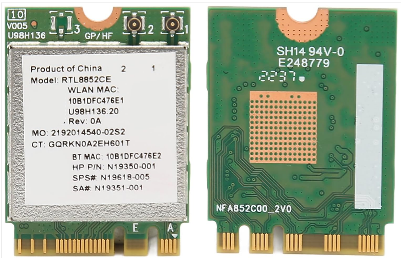
Image 5.1: Front and back views of the ASHATA 6E Card, showing the M.2 connector and component layout for proper installation.
