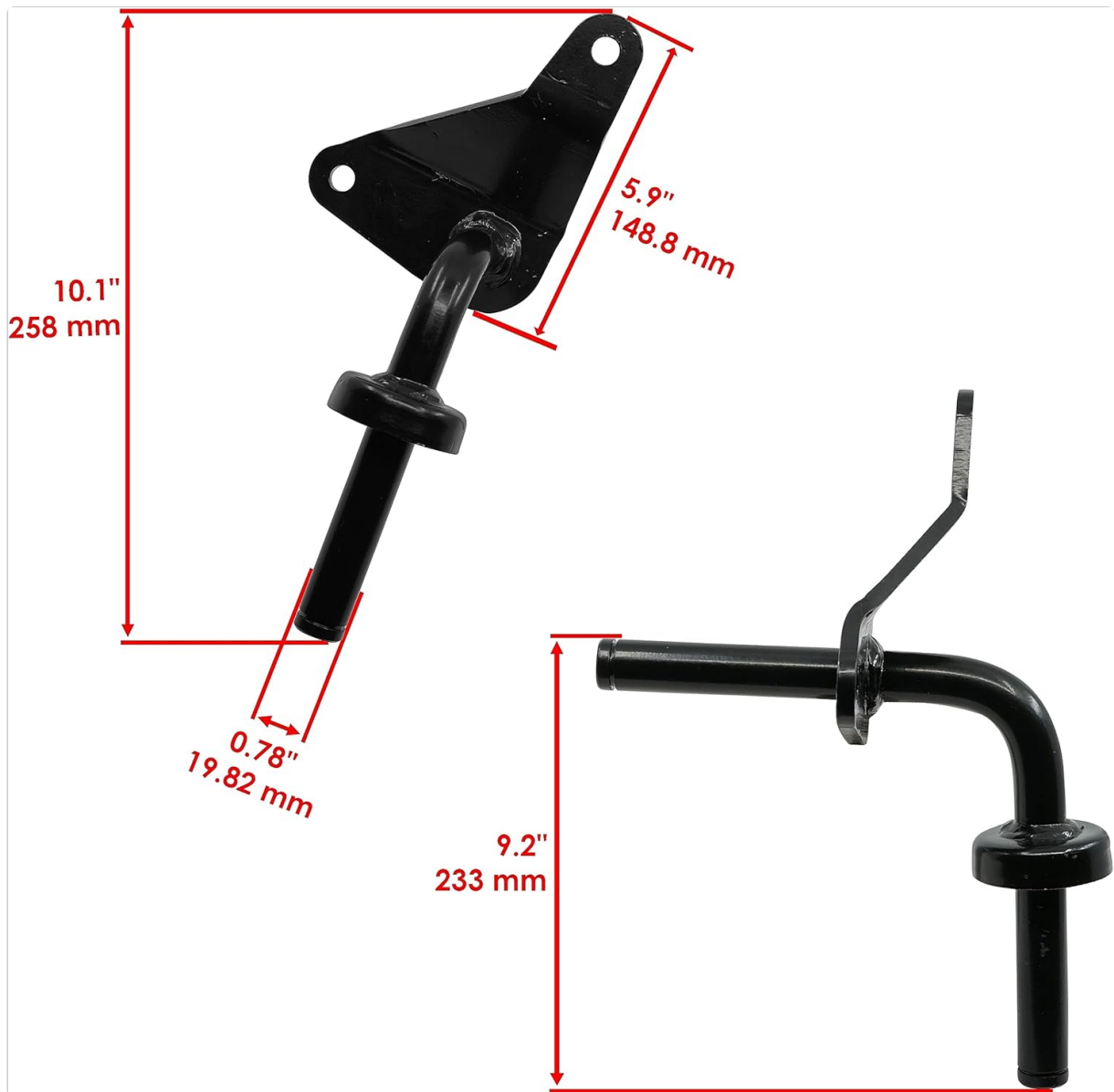
Image 4: Detailed dimensions for the Left Side Spindle Arm.
