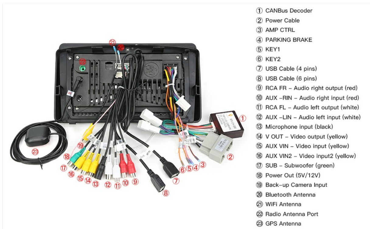
Figure 2: Detailed wiring diagram for the head unit connections.
