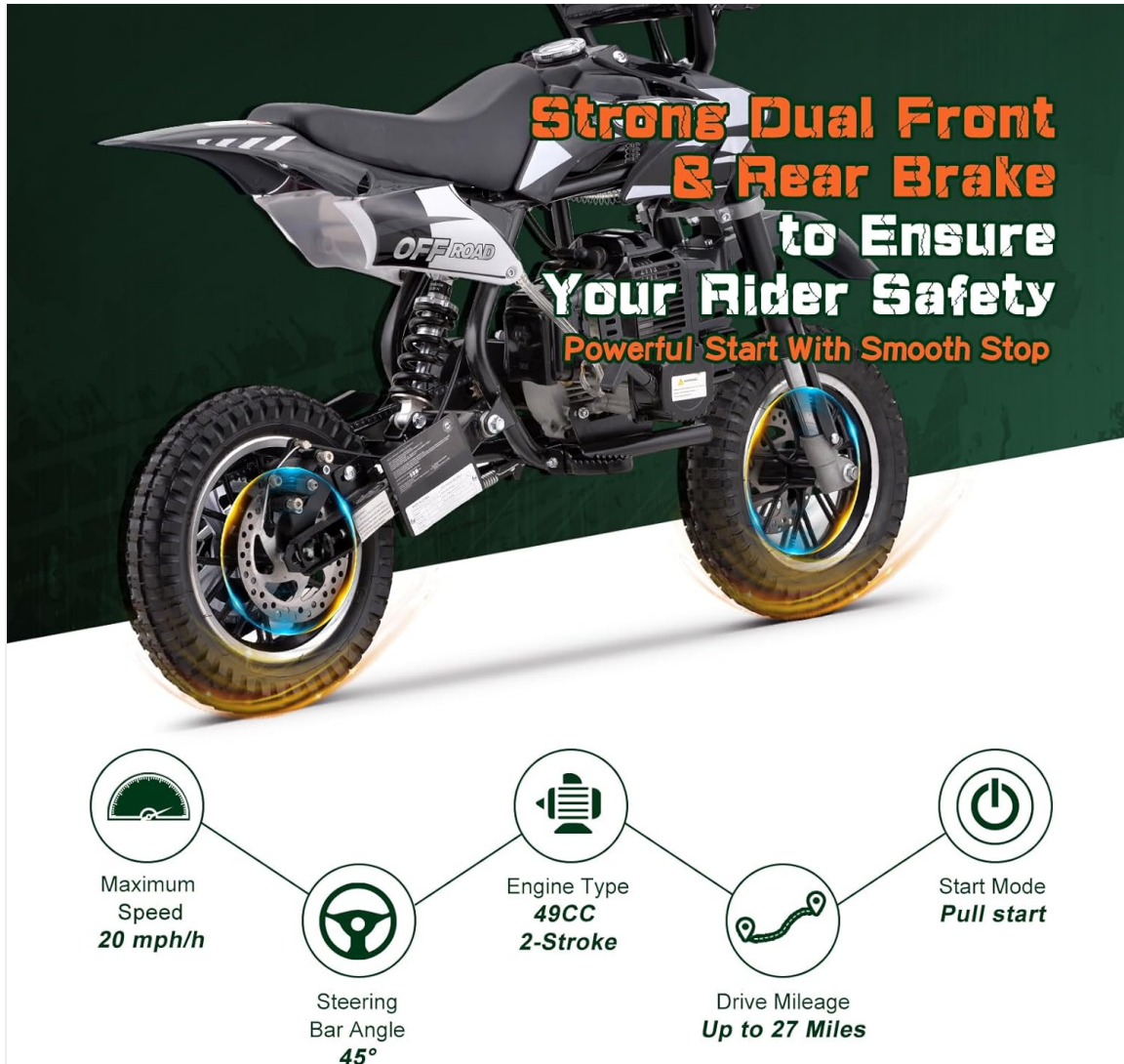
Image 5.1: The dirt bike features strong dual front and rear disc brakes for effective stopping power.
