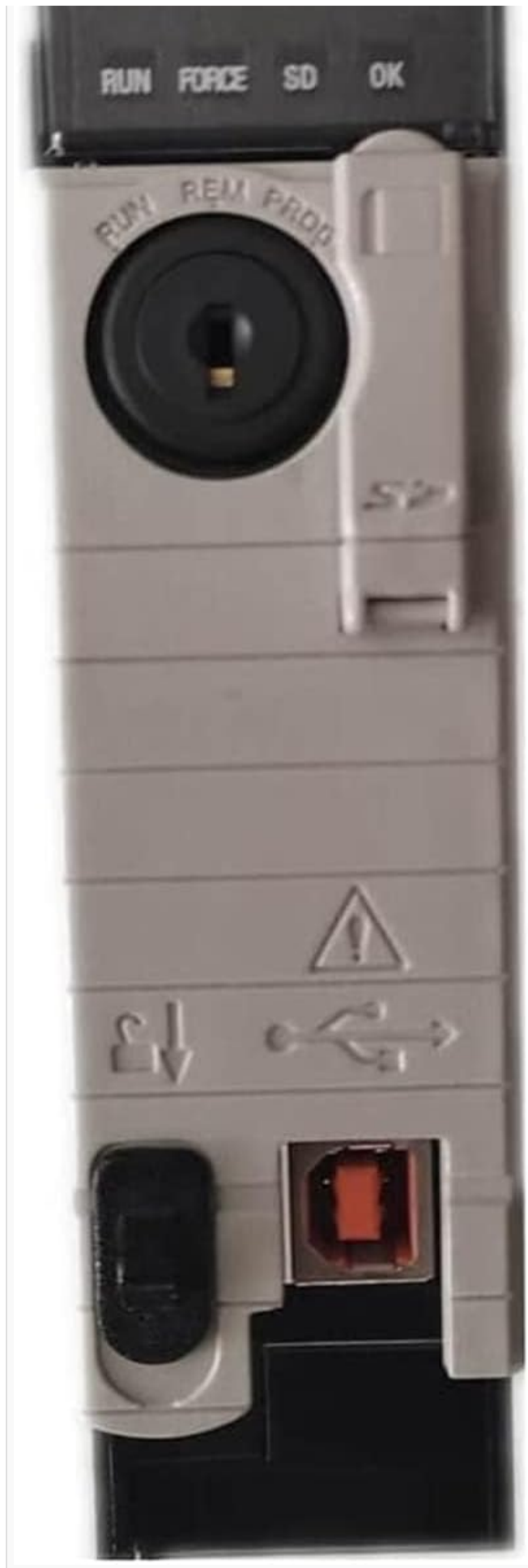
Figure 3.1: Front View of 1756-L75 Module. This image displays the front panel of the Lanlily 1756-L75 Processor Controller Module. Visible features include the 'Logix5575' branding, status indicators (RUN, FORCE, SD, OK) for operational status, a key switch with positions for RUN, REM (Remote), and PROG (Program) modes, an SD card slot for memory expansion or program storage, and a USB port for local connection and programming.
