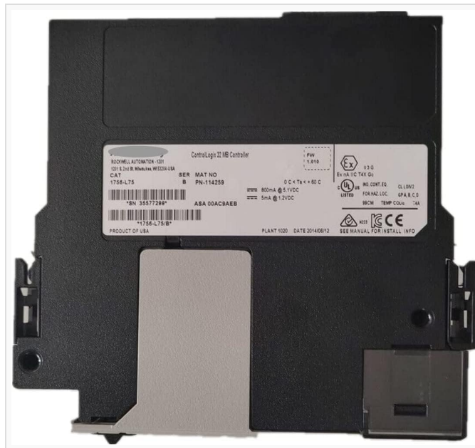
Figure 3.2: Rear View and Product Label. This image shows the rear of the Lanlily 1756-L75 Processor Controller Module, highlighting its product label. The label includes critical information such as 'Rockwell Automation' and 'ControlLogix 32 MB Controller', the model number 'CAT 1756-L75', serial number, firmware version (FW 1.010), power specifications (800mA @ 5.1VDC, 5mA @ 1.2VDC), and various regulatory certifications (UL, CE, Ex).
