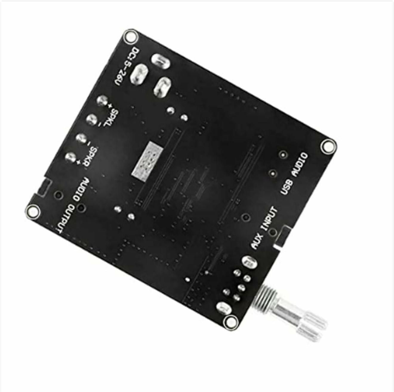
Image 2: Rear view of the XY-C50L amplifier board. This image highlights the connection terminals: DC 5-26V power input, SPKL (Left Speaker) and SPKR (Right Speaker) outputs, AUDIO OUTPUT, USB AUDIO input, and AUX INPUT. The rotary encoder shaft is also visible from this side.
