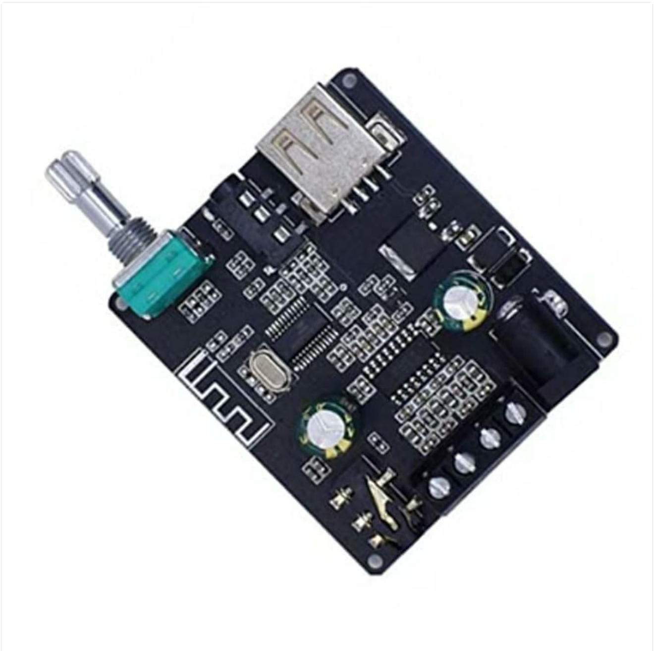
Image 1: Front view of the XY-C50L amplifier board. This image displays the main components visible from the top, including the
