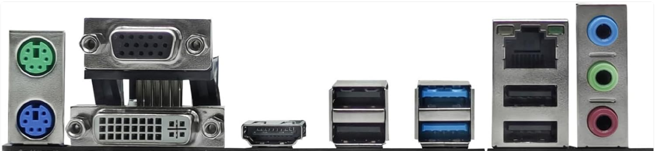
Figure 2.2: Detailed view of the rear I/O panel, showing ports for PS/2, VGA, DVI, HDMI, USB 2.0, USB 3.0, LAN, and audio jacks.
