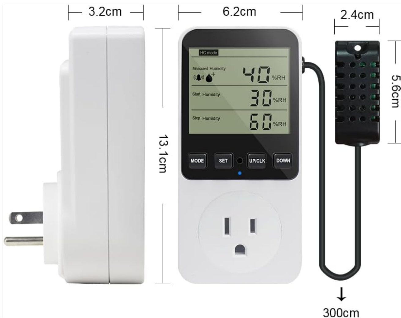
Diagram showing the physical dimensions of the controller and its external sensor, including the sensor cable length.
