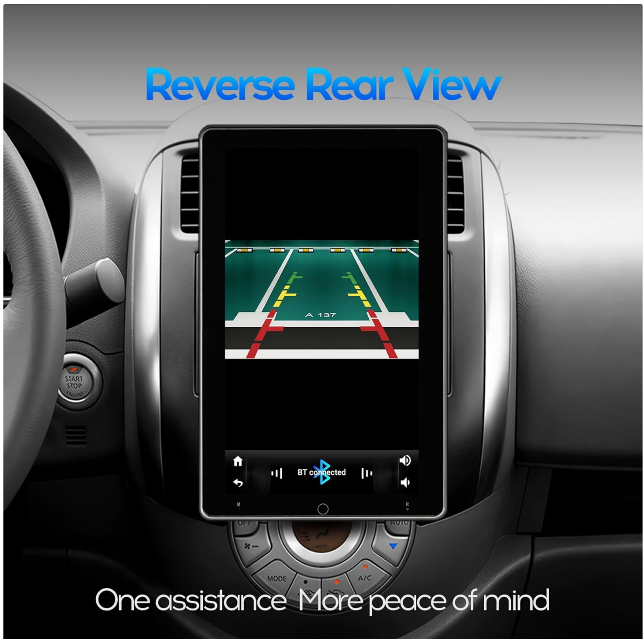
Figure 6.4: Reverse Rear View. This image shows the unit displaying the feed from a rear-view camera, complete with dynamic parking guidelines, assisting with safe reversing.
