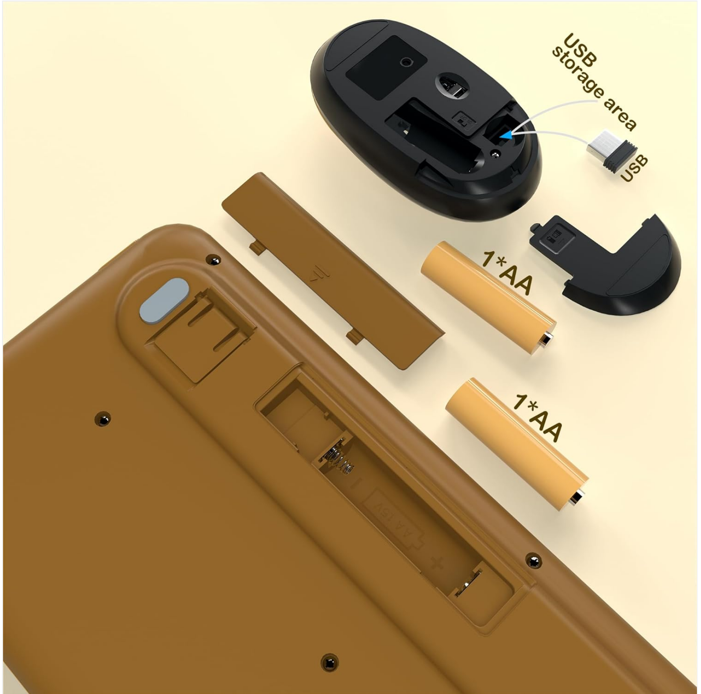
Image 2.1: Illustration of battery installation for both the keyboard and mouse, showing the battery compartments and AA battery placement.
