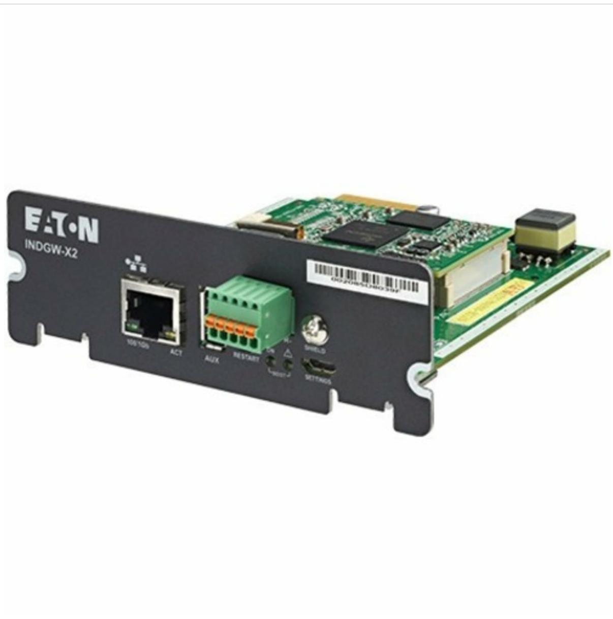
This image displays the Eaton Gigabit Industrial Gateway X2 Card, highlighting its compact design and the available network (RJ-45) and USB ports for connectivity.
