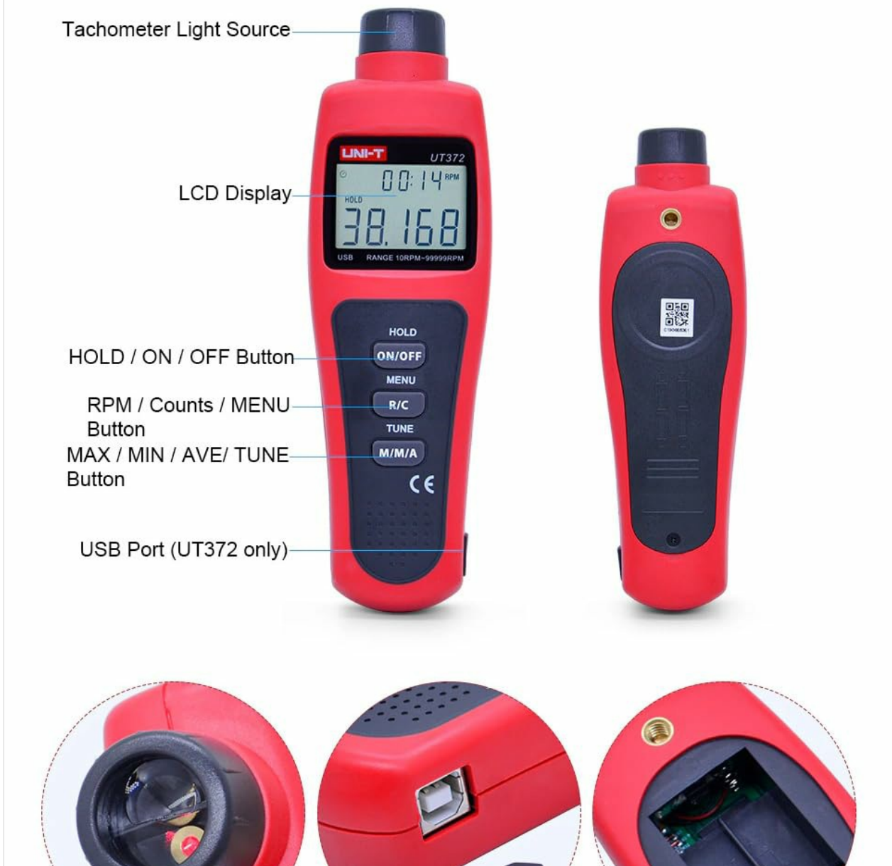
Image 4.1: Front and side view of the UT372 tachometer with labeled components.
