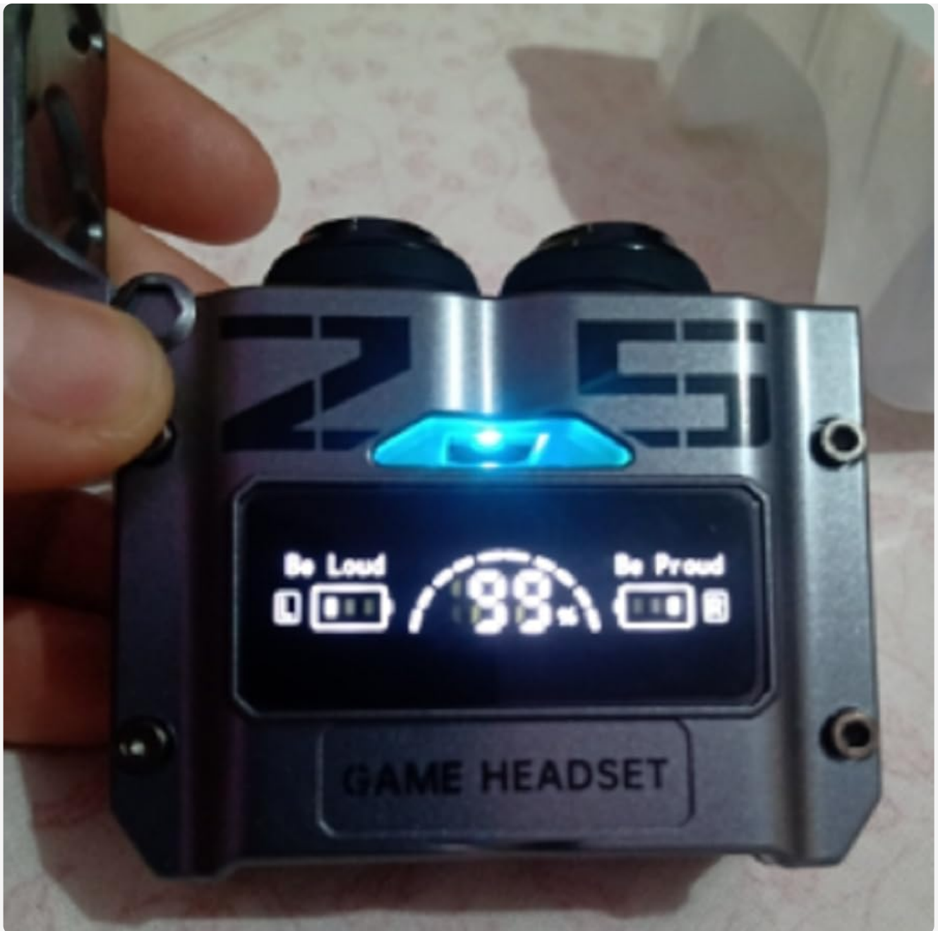
Image 3.3: The M25 charging case with earbuds inserted, showing the digital display. The display indicates the charging status and battery percentage of both the case and the individual earbuds.
