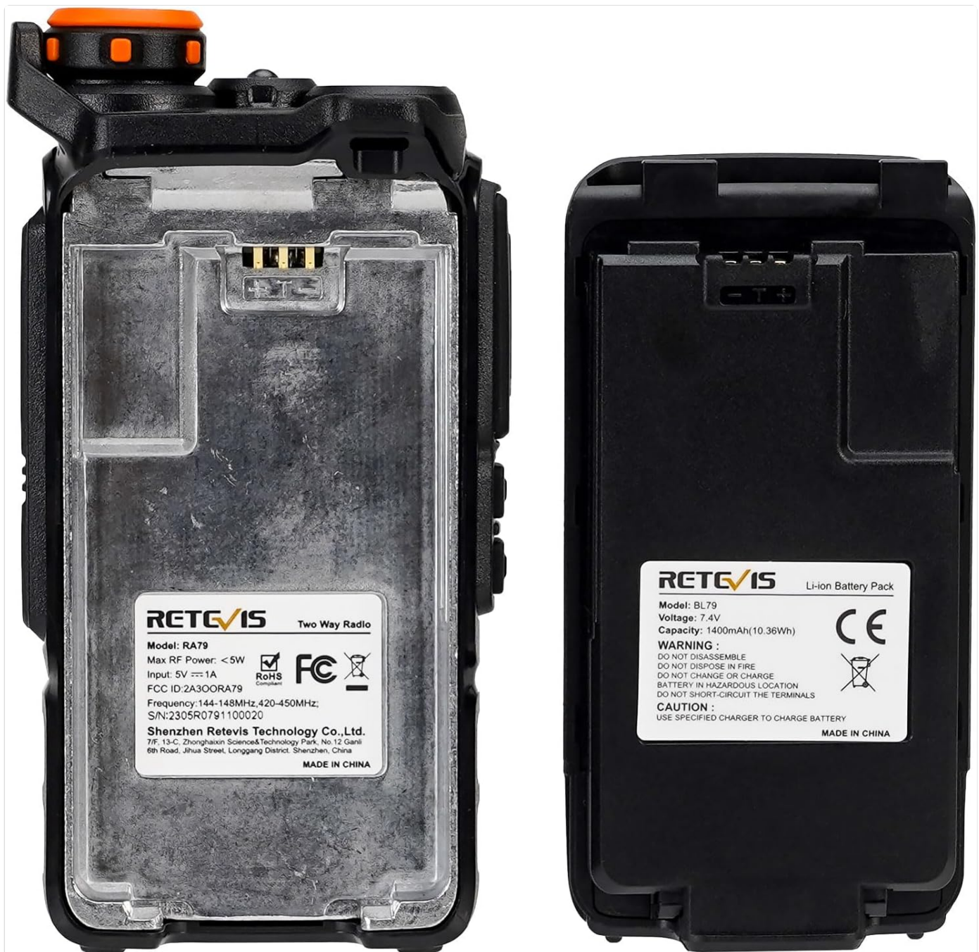
Image: The back of the Retevis RA79 radio and its removable 1400mAh Lithium-Ion battery, showing the contact points.
