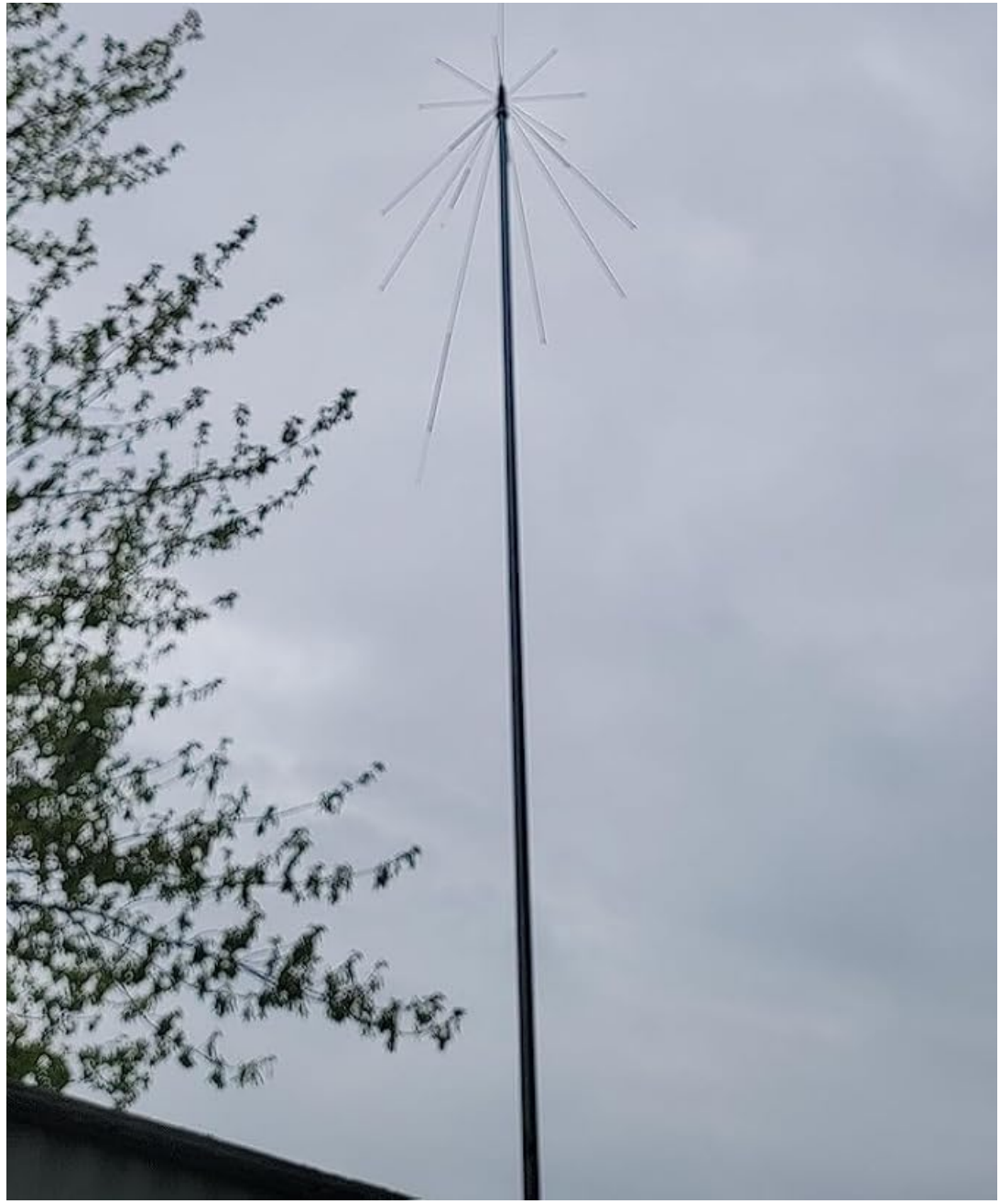
Image: The SIGNALPLUS Discone Antenna installed on a mast, demonstrating a typical outdoor setup.
