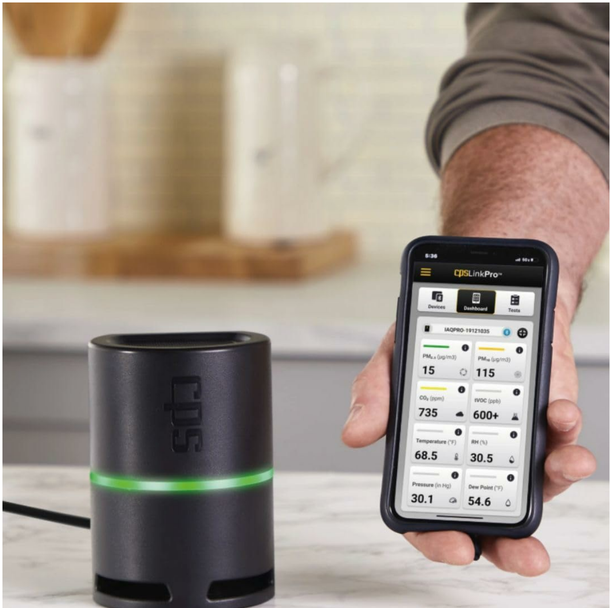
A close-up view of the CPS IAQPRO meter next to a smartphone, showcasing the detailed air quality metrics and comfort zone graph available in the CPSLinkPro app.
