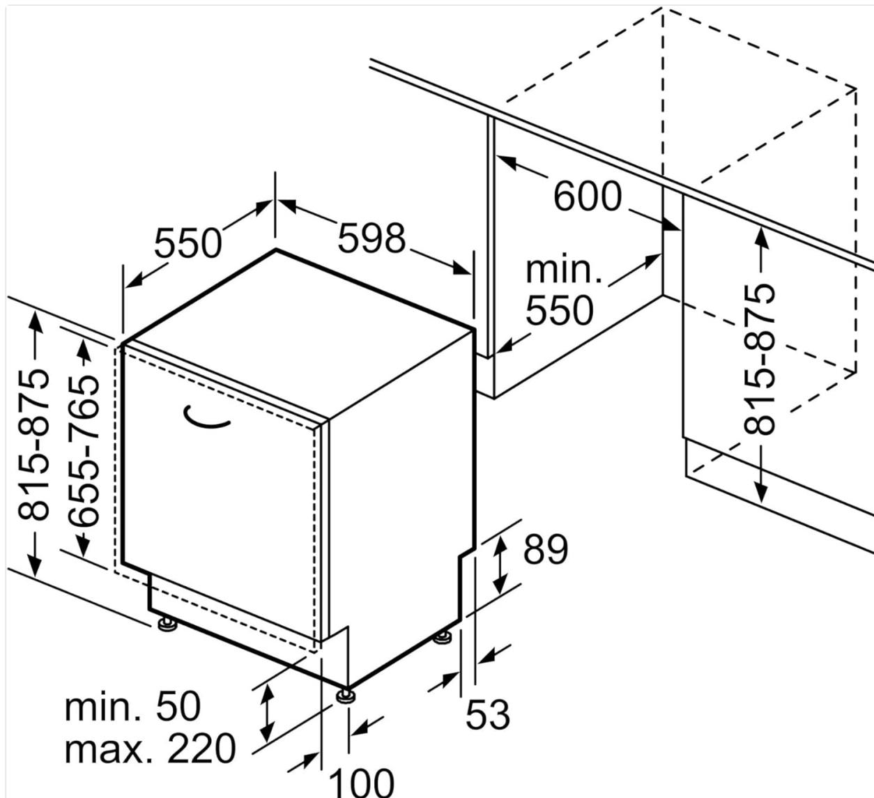
This diagram provides precise measurements for cabinet cutouts and clearances required for proper installation of the dishwasher.
