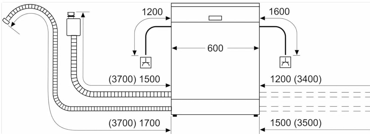
This illustration details the necessary connections for water supply, drainage, and power, crucial for correct dishwasher setup.
