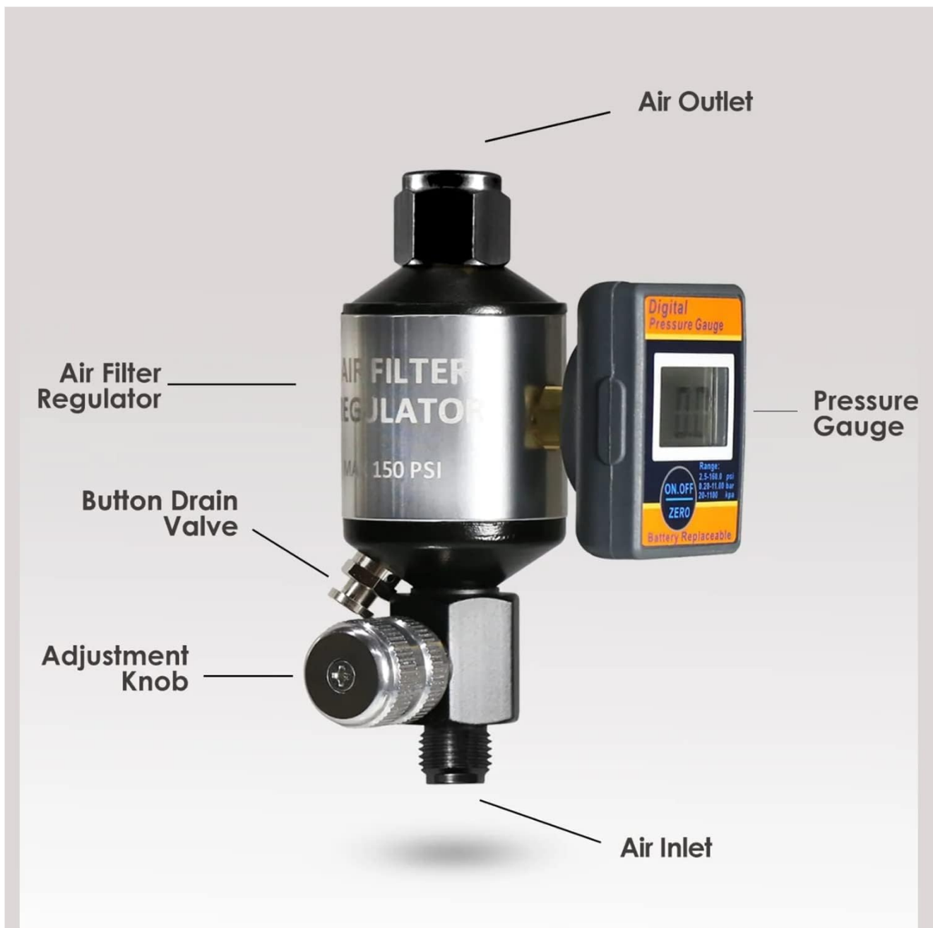
Figure 2: AI303-R2 Digital Air Filter Regulator Components. This image shows the main parts of the AI303-R2 unit, including the air outlet, air filter regulator body, digital pressure gauge, button drain valve, adjustment knob, and air inlet.
