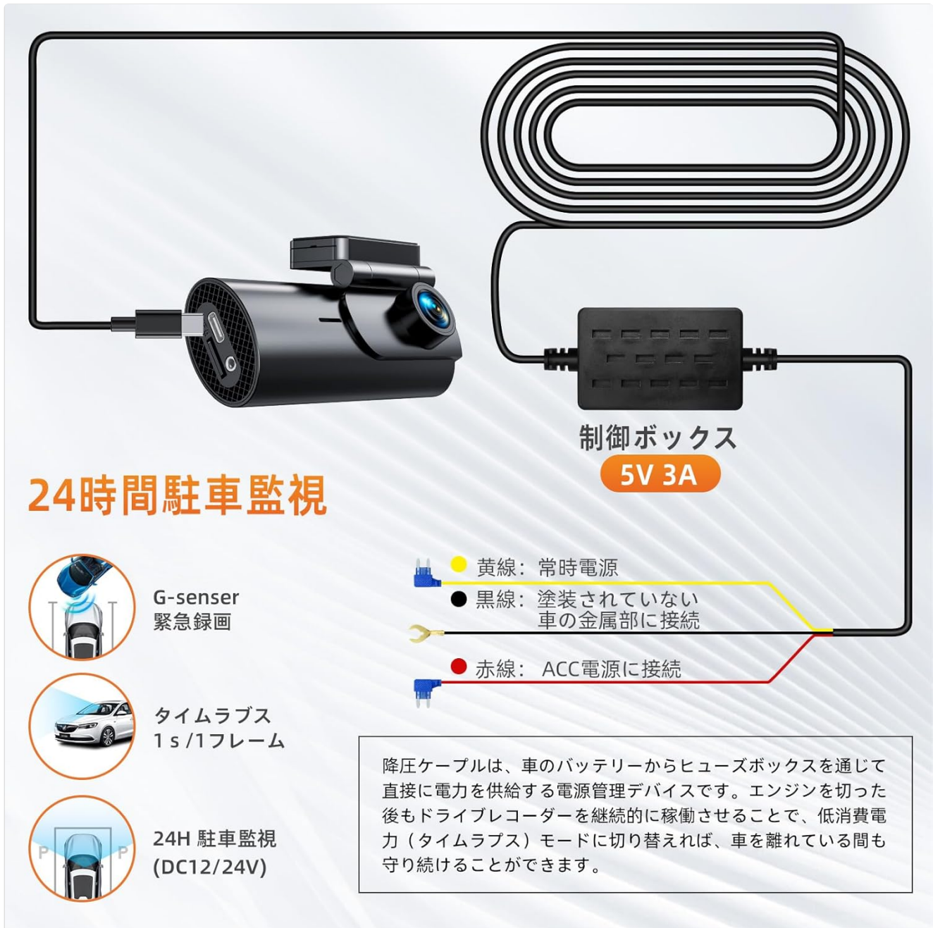
Image 3: Wiring diagram showing connections for the GKU Type-C Step-Down Cable to a dash camera and vehicle's power system. Yellow wire for constant power, red wire for ACC power, and black wire for ground. Illustrates how the cable enables 24-hour parking monitoring features like G-sensor and time-lapse recording.
