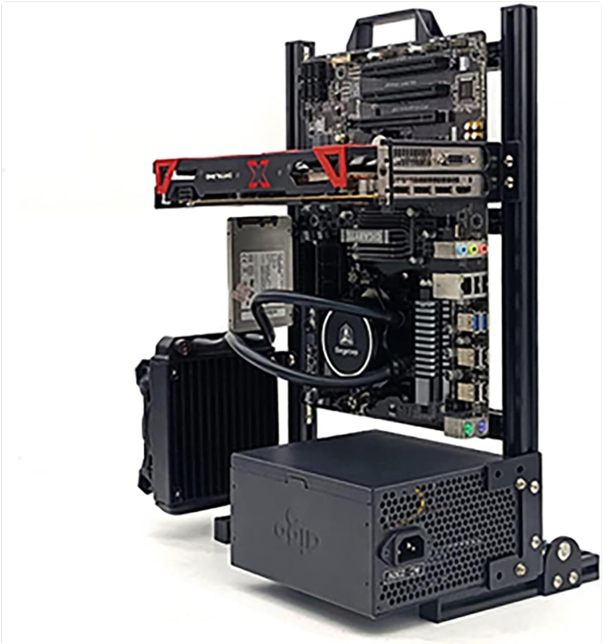
Figure 4.3: Angled view showing a complete setup with power supply and liquid cooling.
