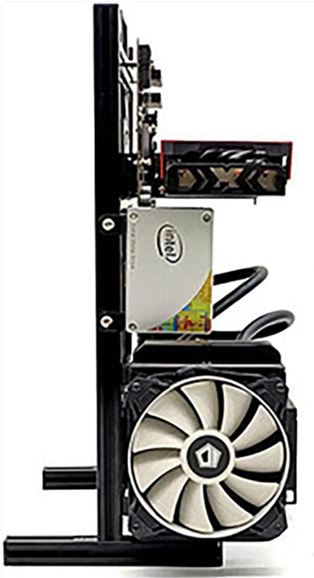
Figure 4.2: Side view of the test bench with a motherboard, graphics card, and AIO liquid cooler installed.
