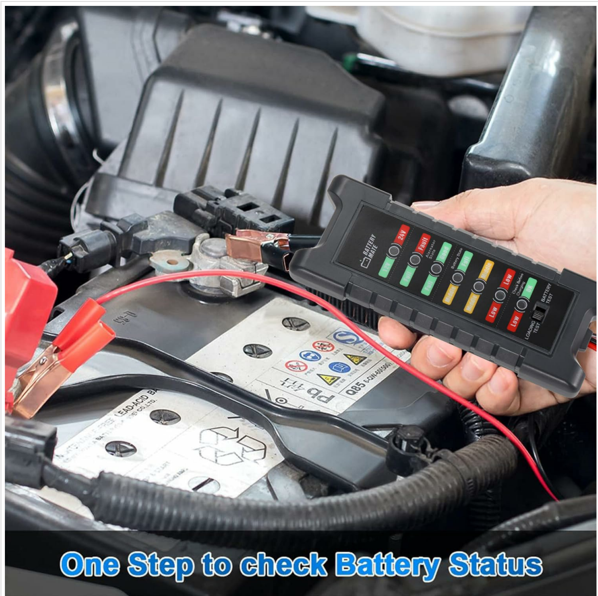
Figure 4.1: Correct connection of the tester to a car battery.
