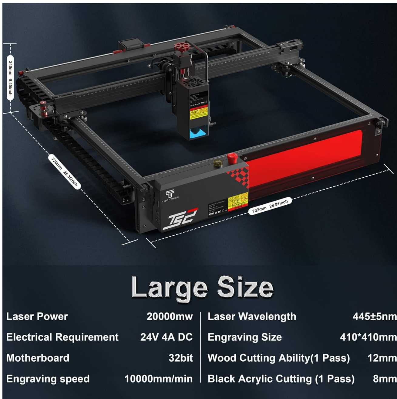
Image 8.1: Dimensional overview of the Twotrees TS2-20W laser engraver.
