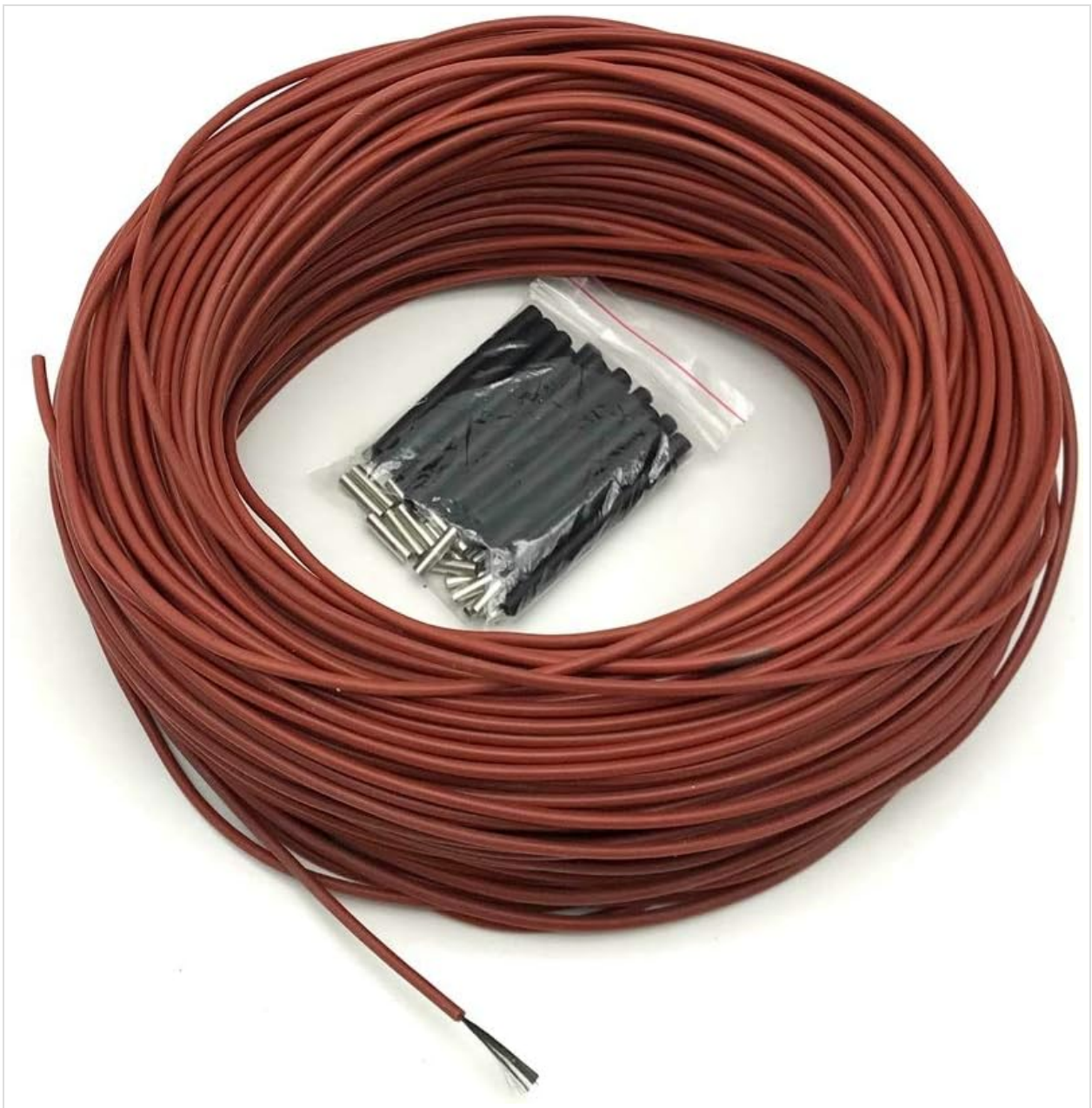
Image: A coil of the 12K 33ohm/m carbon fiber heating cable, along with a bag containing copper crimp tubes and heat shrink sleeves for making electrical connections.
