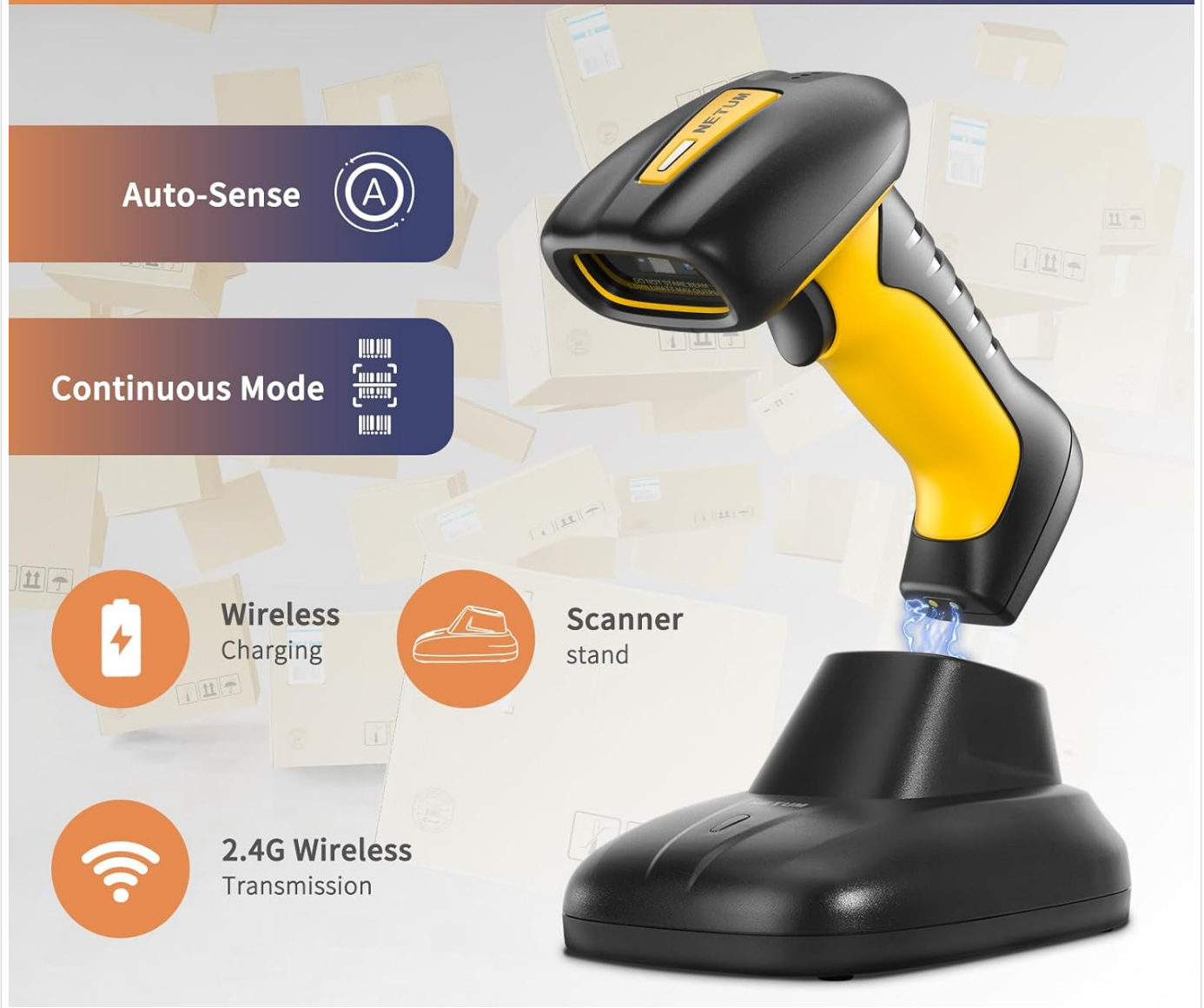
Figure 4.2: The multifunctional cradle serves as a scanner stand, provides wireless charging, and acts as a 2.4G wireless transmission receiver. It supports Auto-Sense and Continuous Mode operations.
