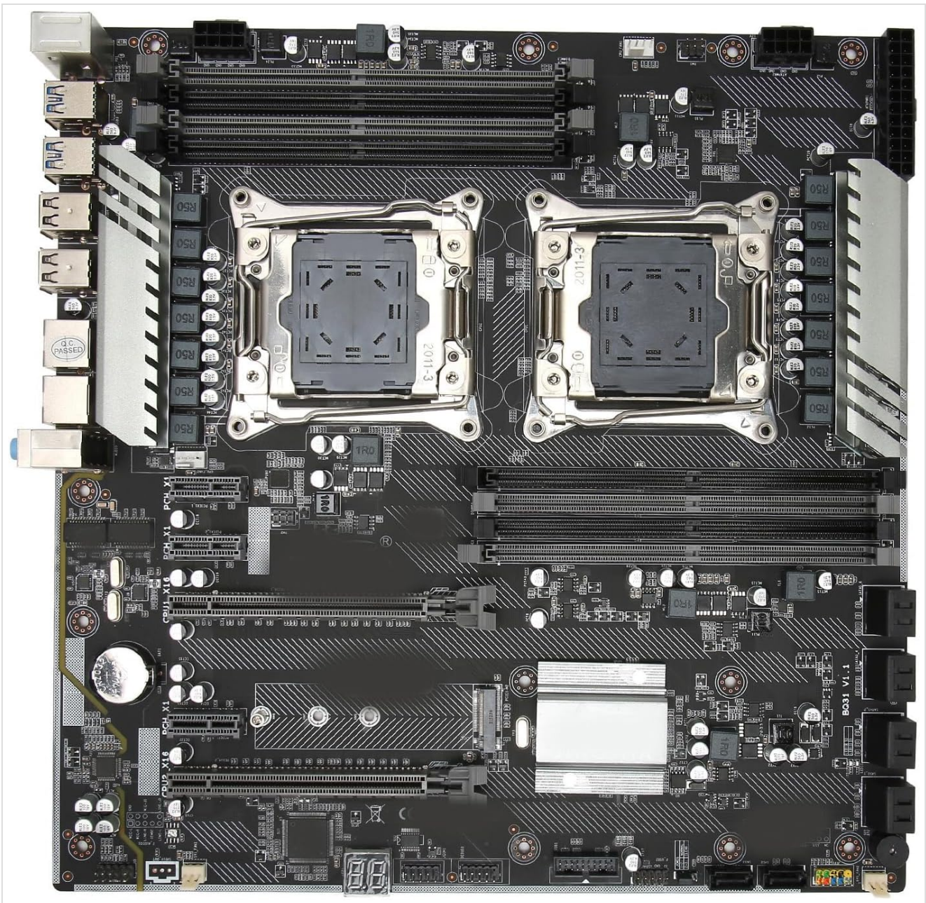
Image: Overview of the Yoidesu X99 F2 E-ATX Motherboard, showing the dual CPU sockets and memory slots.
