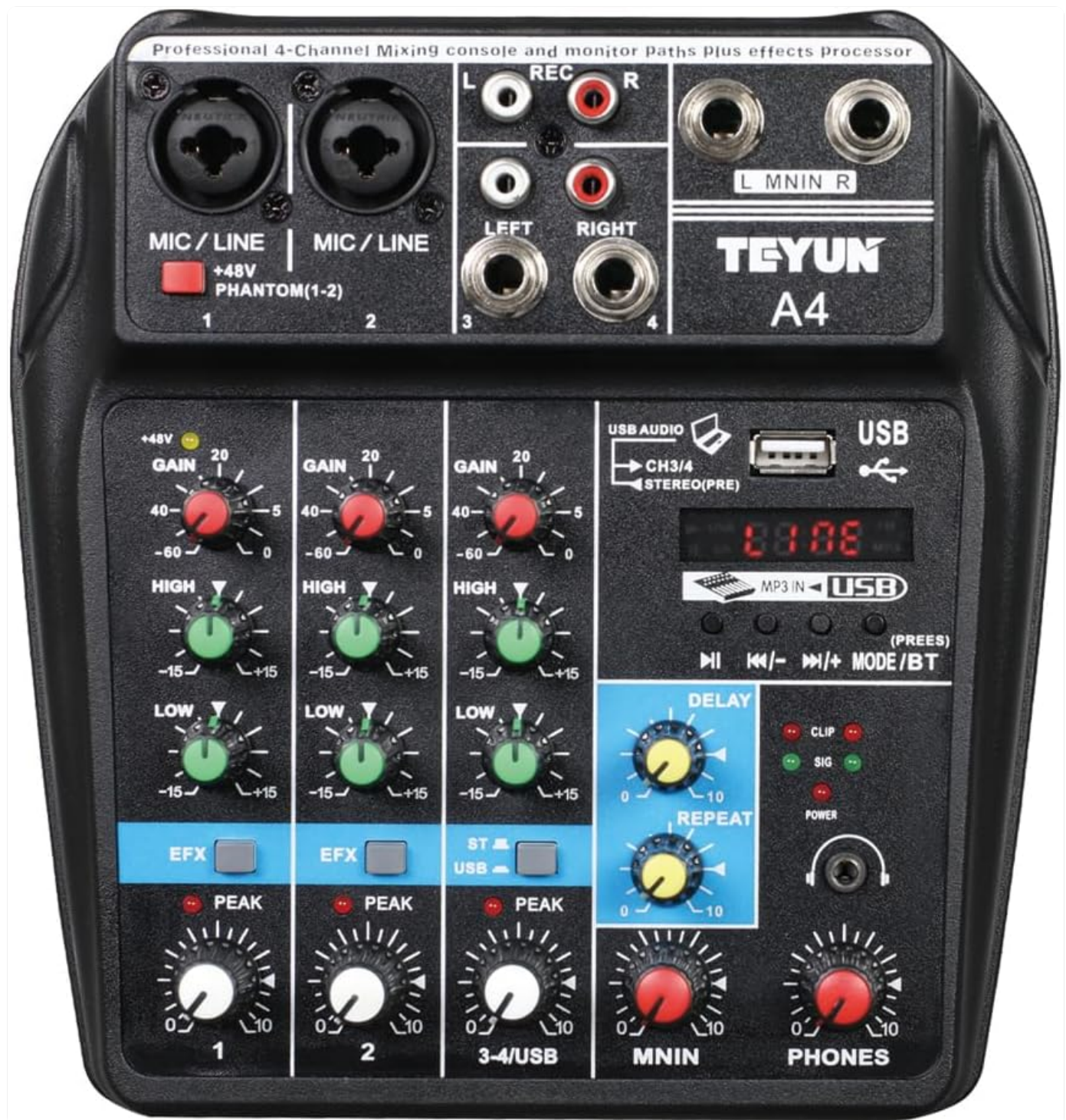
Figure 4.1: TEYUN A4 Control Panel
