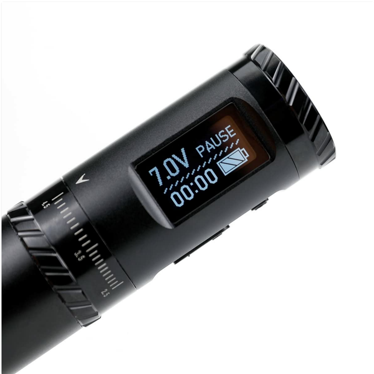
Image 7.2: The OLED display indicating "PAUSE" mode, along with voltage and session time. Note: Image shows a black pen, but display functions are identical.
