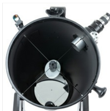
Image: An internal view of the telescope, highlighting the primary mirror and its support structure.
