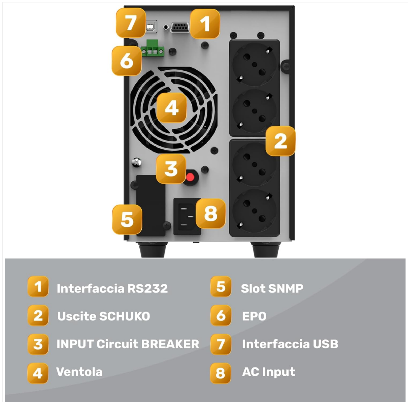
Figure 3.1: Rear panel of the NJOY Echo Pro 2000 UPS, showing various connection ports.
