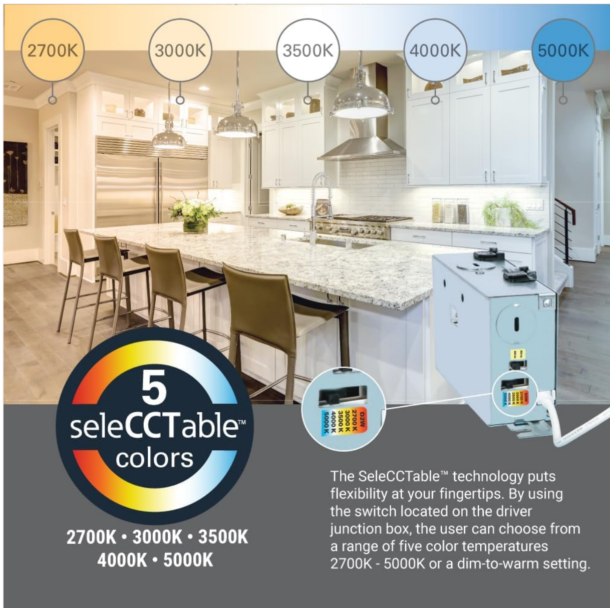
Image: Illustration of the 5 selectable color temperatures (2700K, 3000K, 3500K, 4000K, 5000K) and the switch on the driver junction box for selection.
