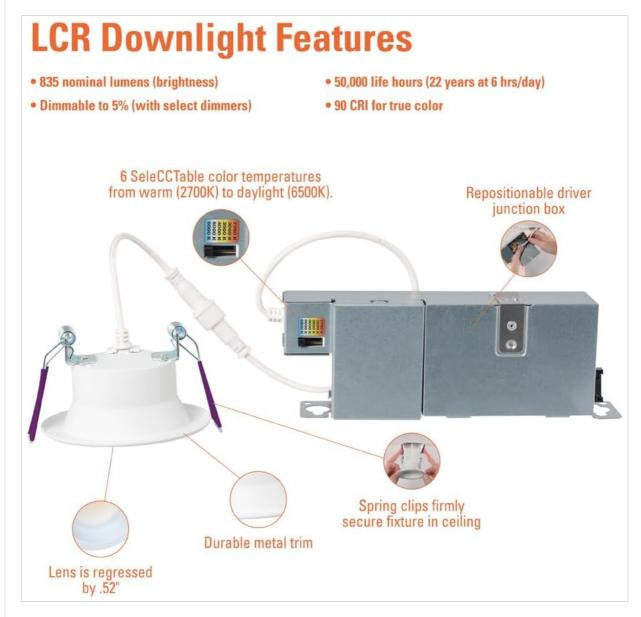
This diagram details key features: 835 nominal lumens, dimmable to 5%, 90 CRI for true color, 6 selectable CCTs (2700K-6500K), repositionable driver junction box, and spring clips for secure ceiling installation. It also shows the lens is regressed by 0.52 inches.
