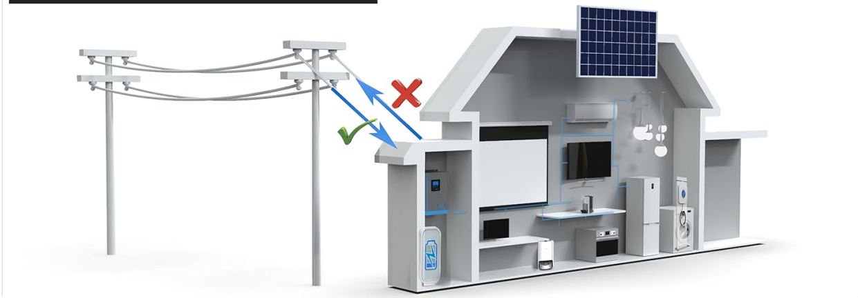
Image: Diagram illustrating the off-grid functionality, showing power flow from solar and battery to home loads without connection to the utility grid.
