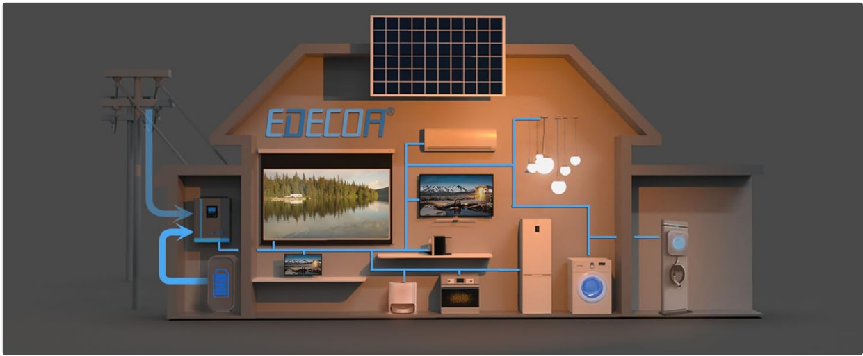
Image: Diagram illustrating the system operating in grid priority mode, where grid power is the primary source, with solar and battery as backup.
