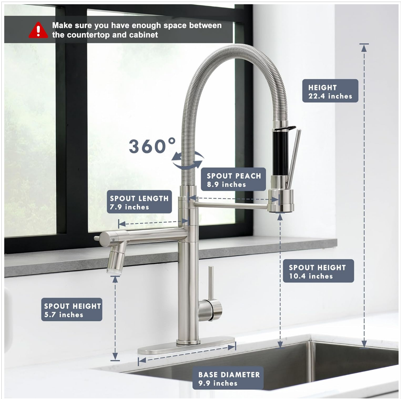
Figure 1: Detailed dimensions of the GIMILI Dual-Spout Kitchen Faucet. Note the 22.4" overall height.
