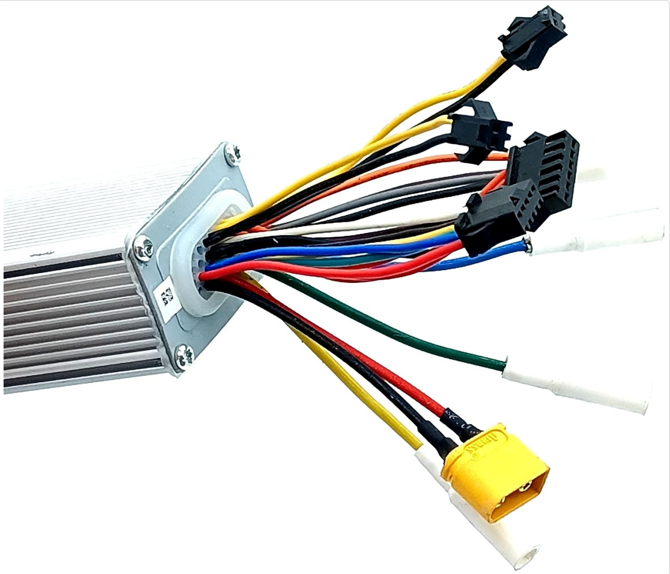
Figure 2.3: Detailed view of the wiring harness, showing the individual wires and their protective sheathing as they emerge from the controller housing.
