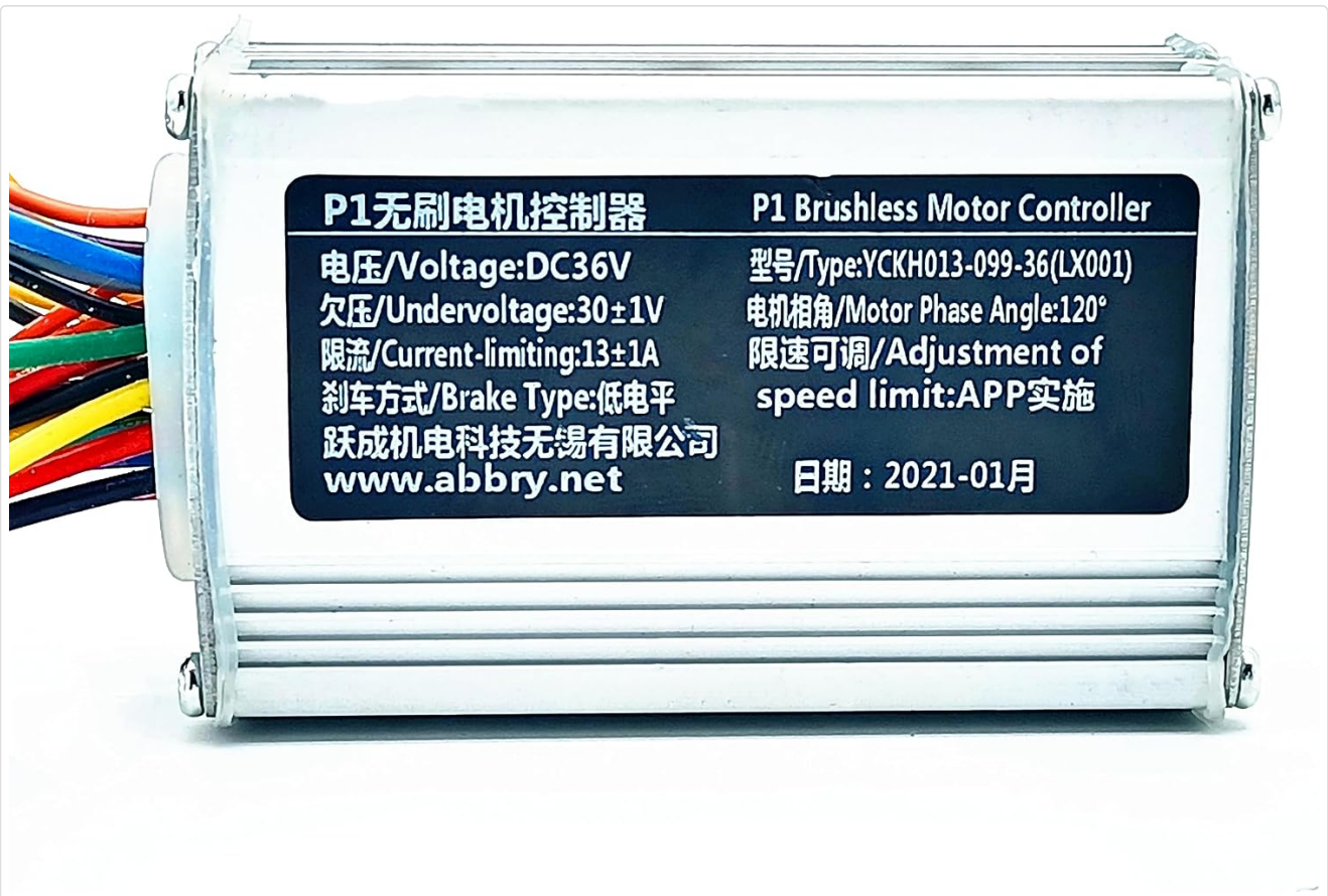
Figure 2.4: Close-up of the product label, displaying key specifications such as voltage, undervoltage, current limit, motor phase angle, and model type.
